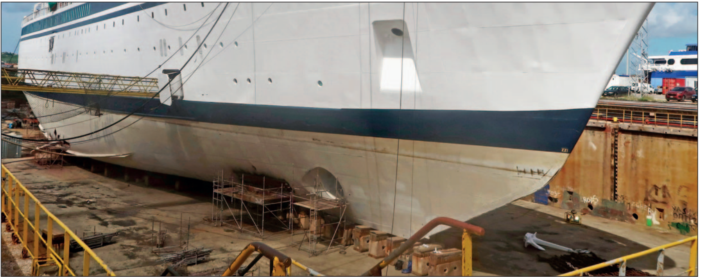
Hull of a small cruise ship with the original Ecospeed coating intact 10 years after application.
