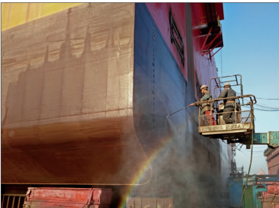
The FLNG Eemshaven being washed down in drydock 7 years after Ecolock was originally applied.
