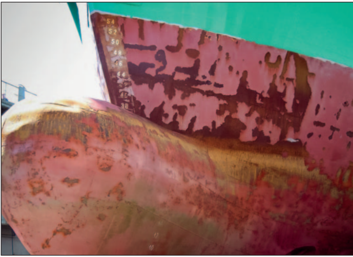
Bulbous bow of a Baltic ice-trading cargo ship in drydock in very poor condition after sailing with conventional antifouling, and same ship after a year of sailing in the same conditions after Ecospeed was applied.
