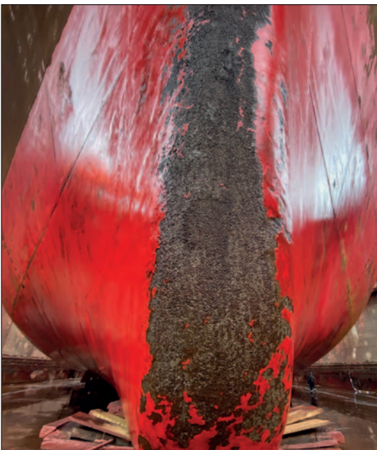
Heavy pitting on the bow of one of the world's most powerful icebreaking cargo ship. The second photo shows the same bow after 3 seasons in the ice, now protected with Ecospeed.
