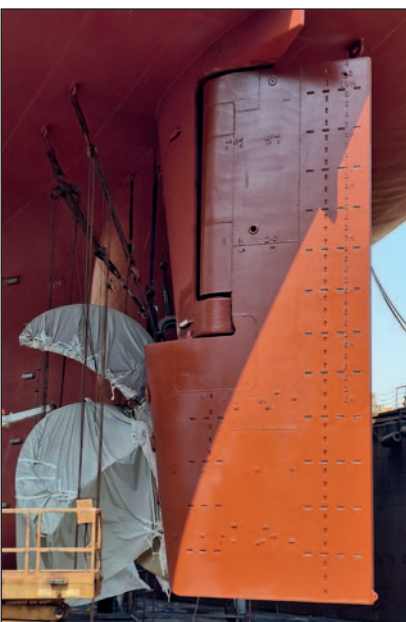
Many customers have reported that they do not need to use cathodic protection on rudders coated with Ecoshield.
