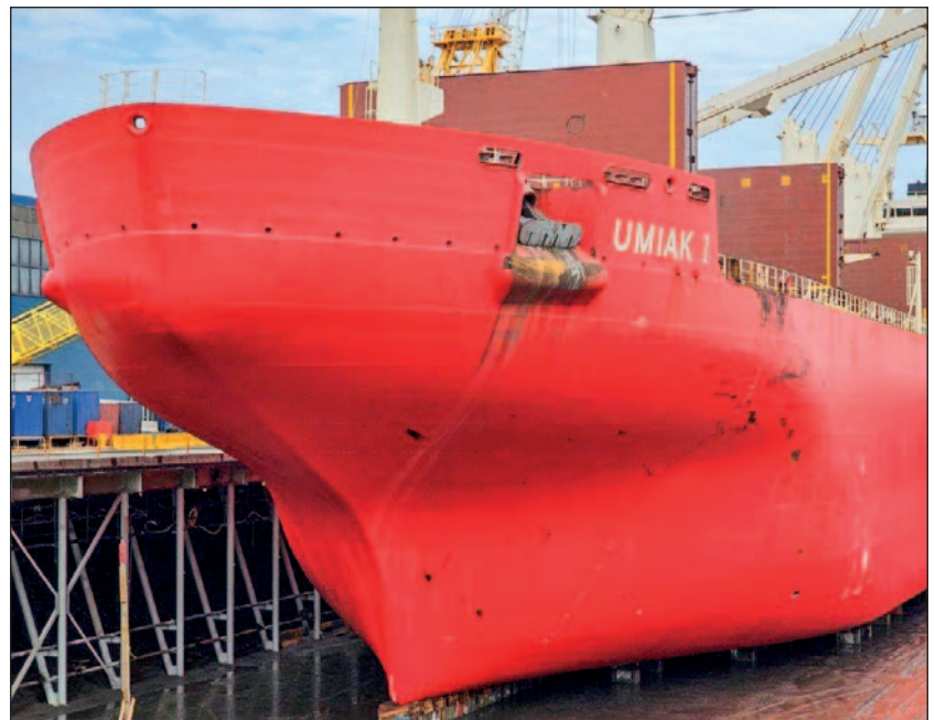
Heavy pitting on the bow of one of the world's most powerful icebreaking cargo ship. The second photo shows the same bow after 3 seasons in the ice, now protected with Ecospeed.
