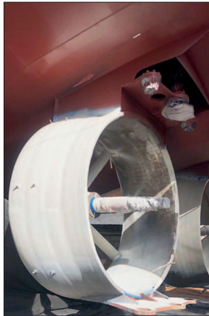
Propeller nozzles after application of first Ecoshield layer.
