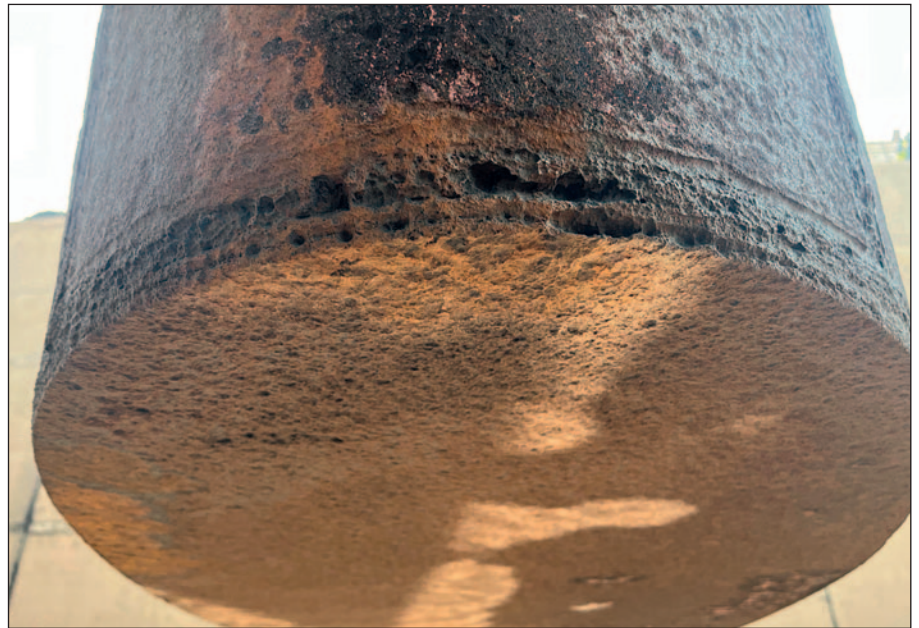
Severe pitting in rudder as a result of cavitation. Ecoshield can prevent this from happening again.
