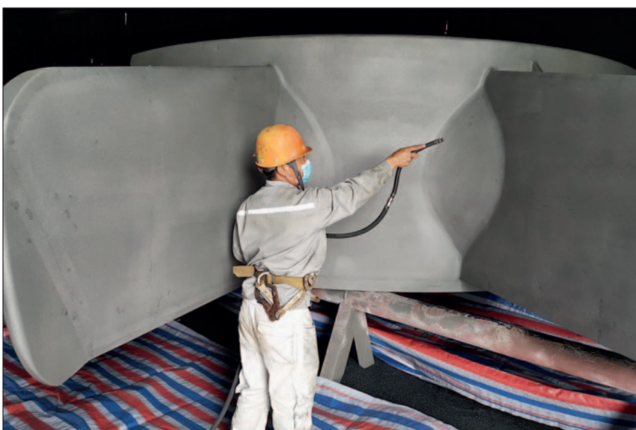
Surface preparation on energy saving device prior to Ecoshield application.
