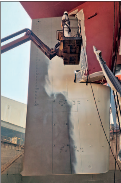
Ecoshield is applied in only two, identical layers.
