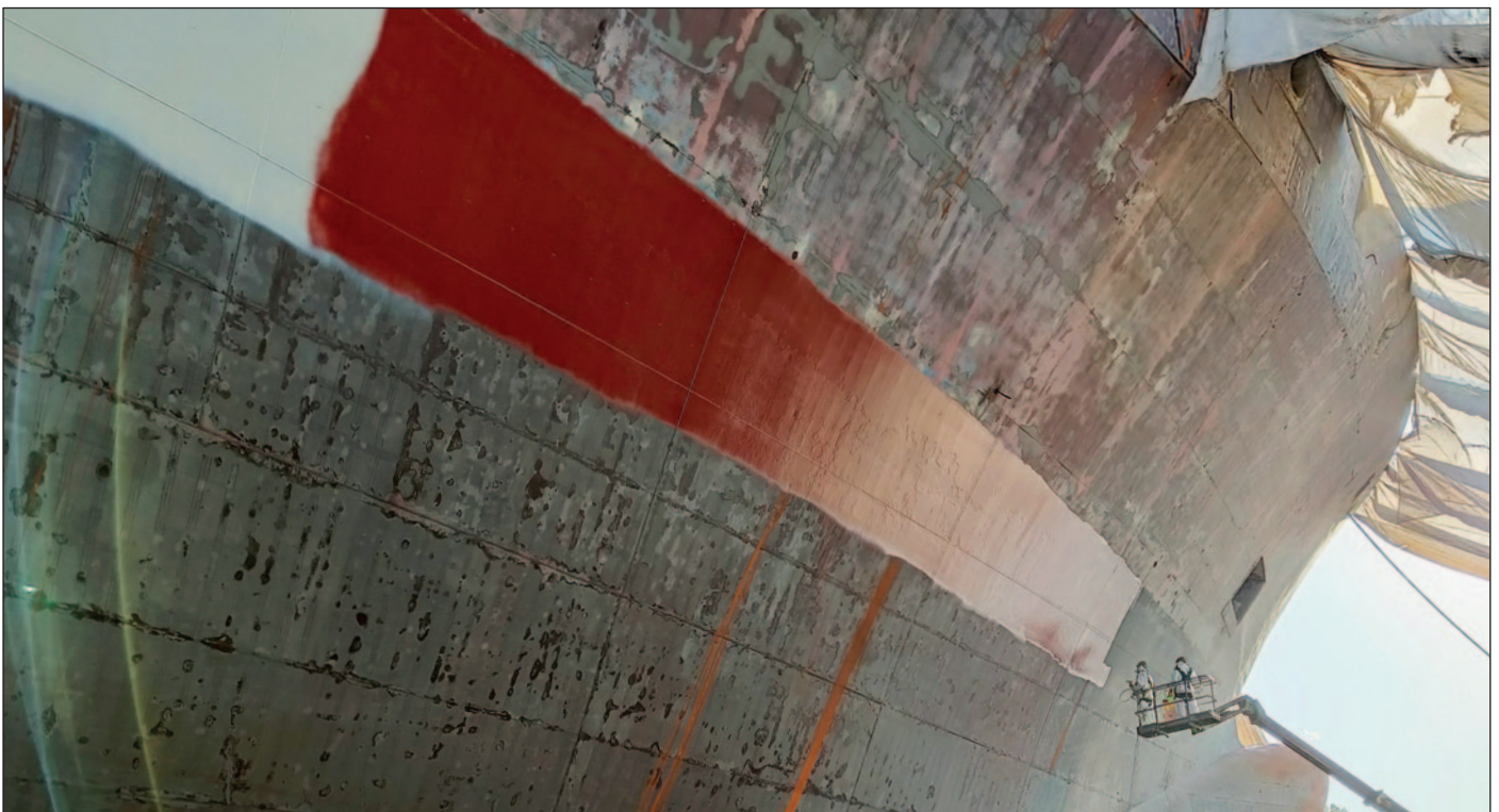
Boottop of container ship being protected with Ecospeed, chosen for its toughness and abrasion resistance.
