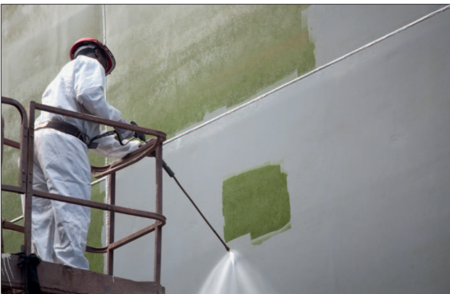
Ecospeed can also be pressure washed in drydock without harm to the coating.
