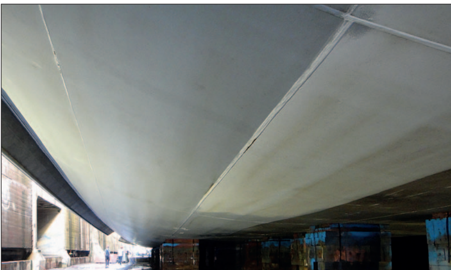
Hull of the same cruise ship in drydock 5 years after Ecospeed was applied, with no recoating, just washed off in drydock.
