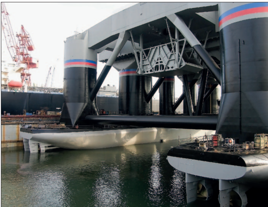
This converted semisubmersible rocket launch platform would lie idle for months and accumulate heavy fouling. This was easily cleaned off when it was time to sail to the equator for the next launch.
