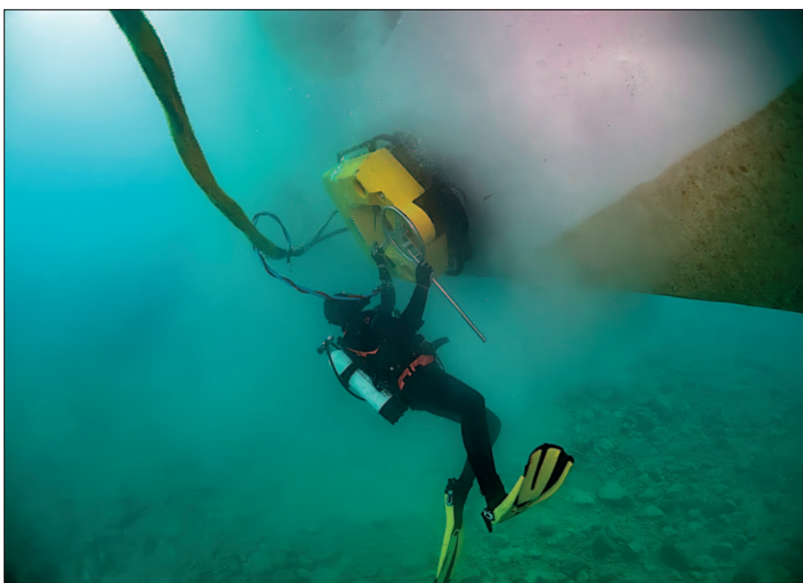
Cleaning the hull of a 340m cruise ship can be accomplished quite rapidly by a competent diver using the Typhoon M313 cleaning unit on Ecospeed coating.
