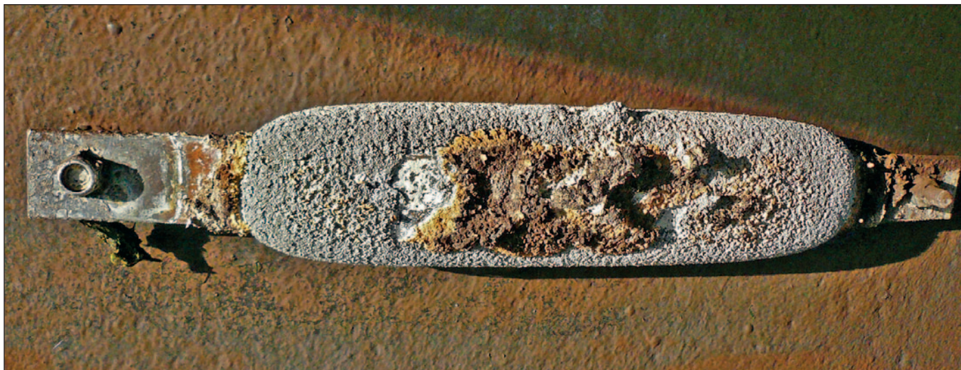
A sacrificial anode is designed to corrode instead of the surface it's attached to.
