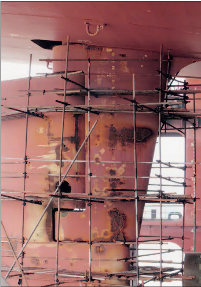
Rudder of large container ship after 5 years of sailing with regular antifouling coating on rudder, showing severe cavitation damage.
