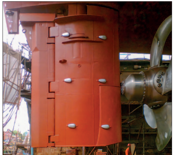
Rudder of same Roro ship protected with Ecoshield for life. Anodes are compatible but not needed.
