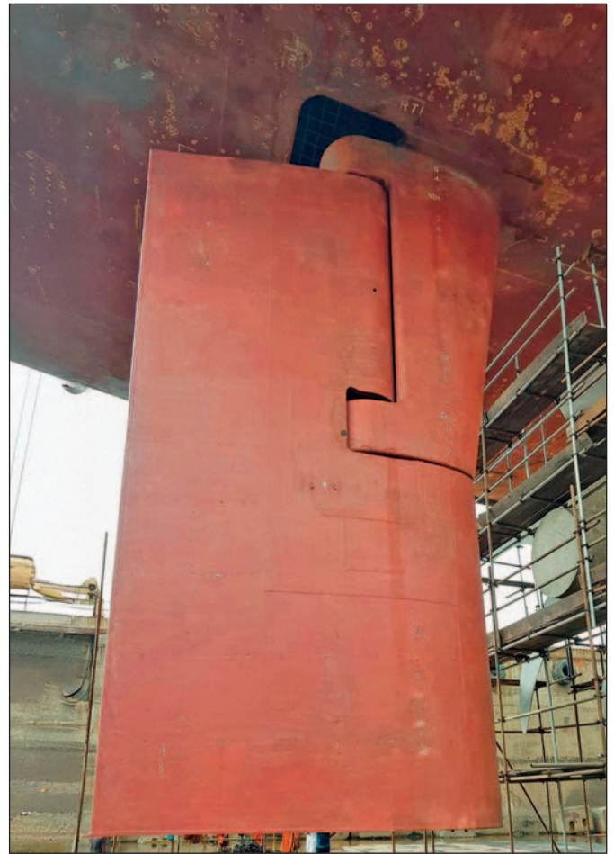
Same rudder of same ship after sailing for 10 years protected with Ecoshield, no repaint, no anodes.
