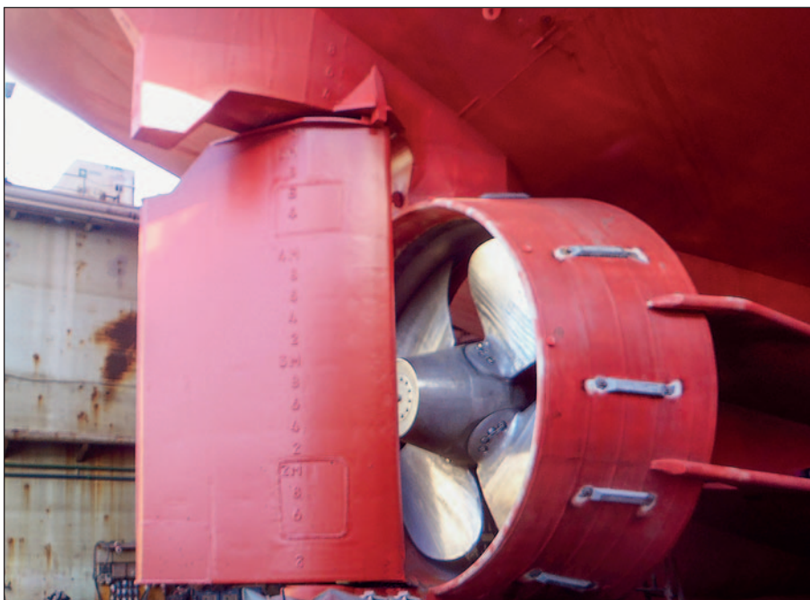
Full spade rudder and nozzle protected with Ecoshield for life.
