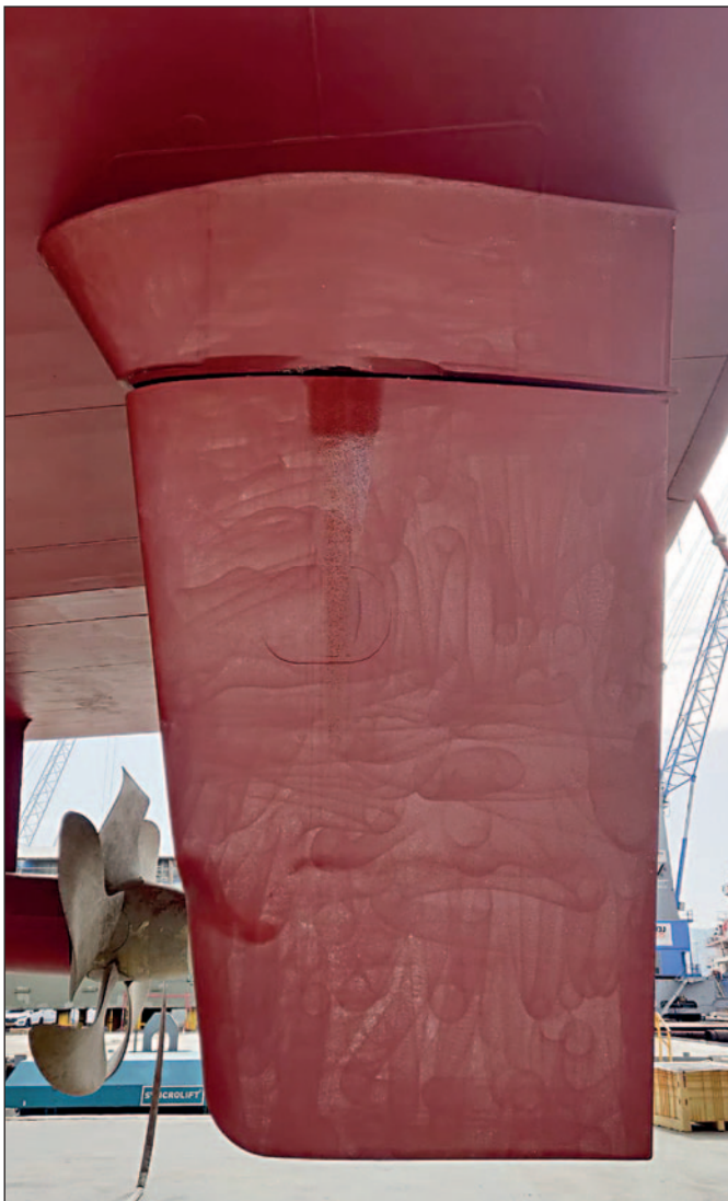
Rudder of fast naval ship protected with Ecoshield, no anodes. Regular hull coating would have disappeared long since.
