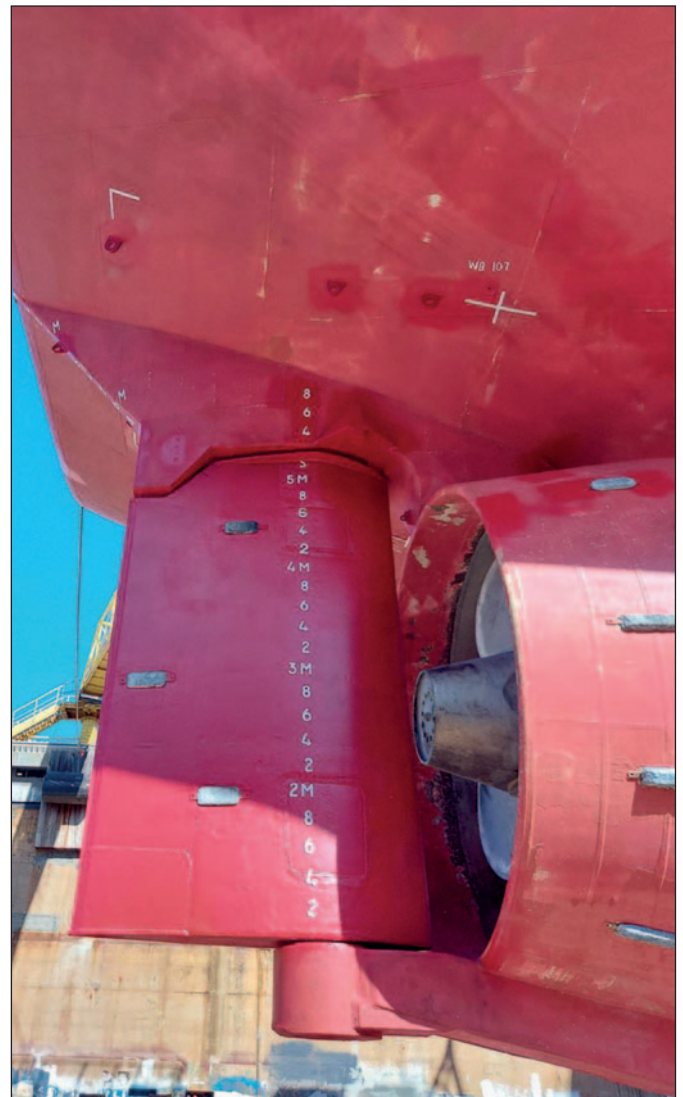
The stern area of an icebreaker showing several anodes in place. Since the hull is coated with Ecospeed, the cathodic protection is not in fact needed.
