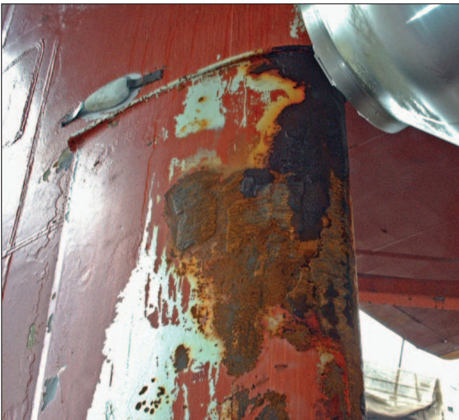
Rudder of Roro ship "protected" with regular antifouling hull coating.
