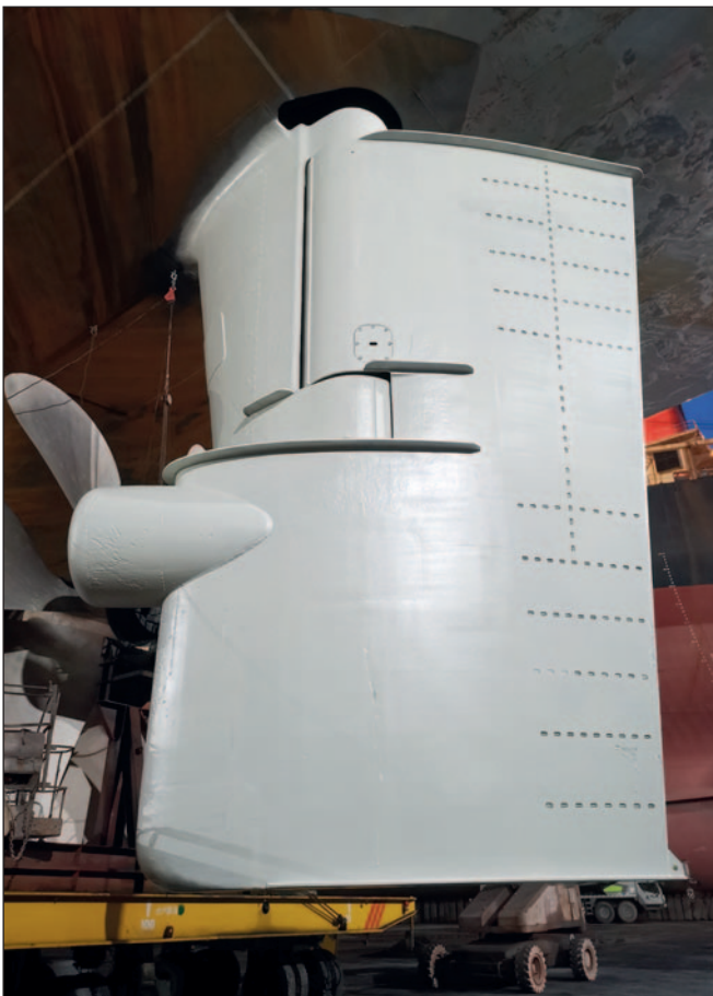
Ecoshield is applied in only two, identical layers.
