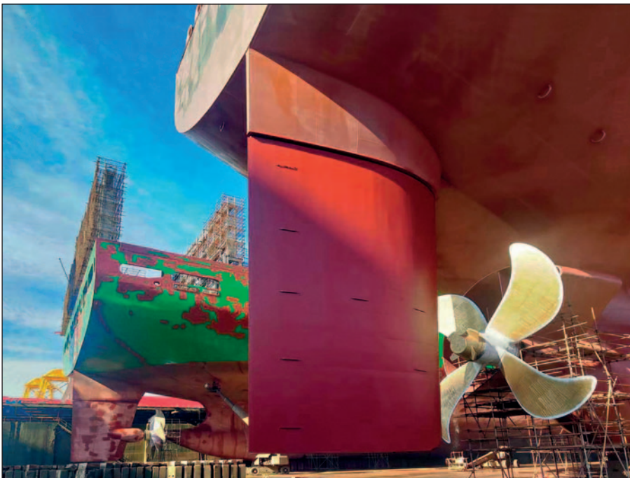
Both Ecoshield layers can be applied very fast, with only three hours in between.
