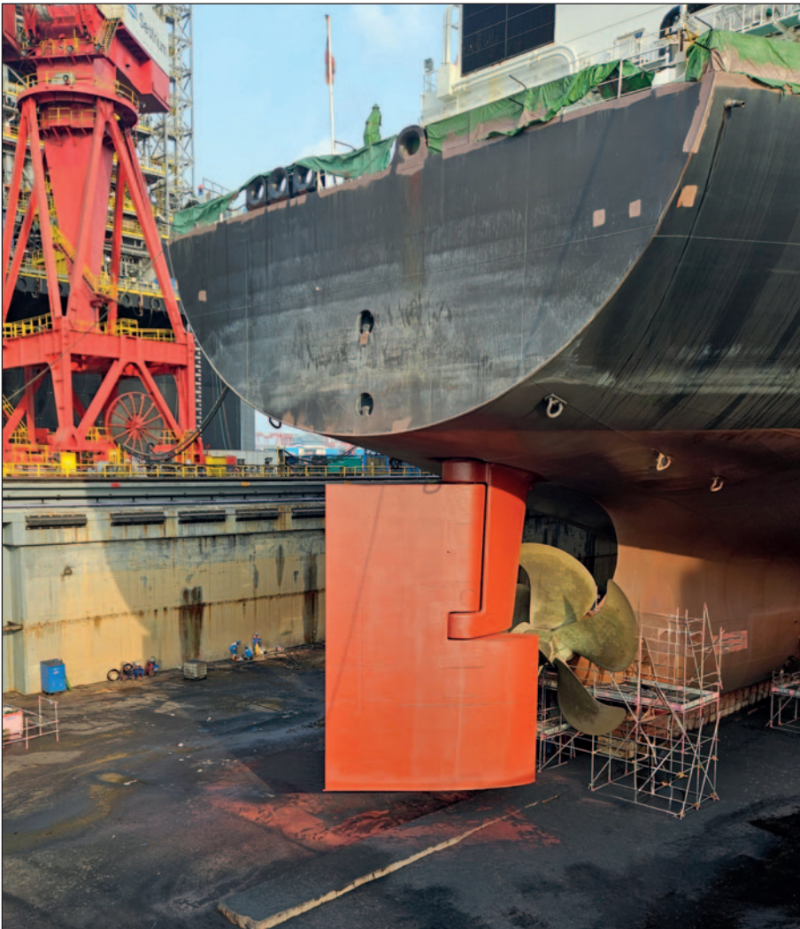
Many customers have reported that they do not need to use cathodic protection on rudders coated with Ecoshield.
