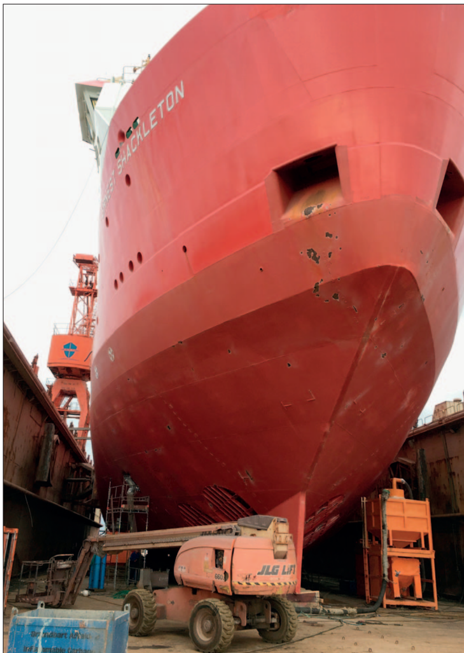
Since the RRS Ernest Shackleton was coated with Ecospeed in 2009, only those areas most susceptible to ice impact have needed minor touch-ups.
