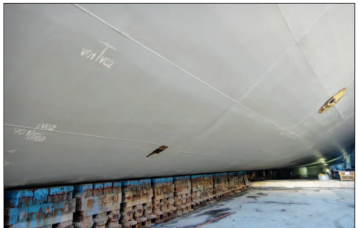
Hull of cruise ship 5 years after being coated with conventional antifouling paint (left) and five years after being coated with Ecospeed (right).
