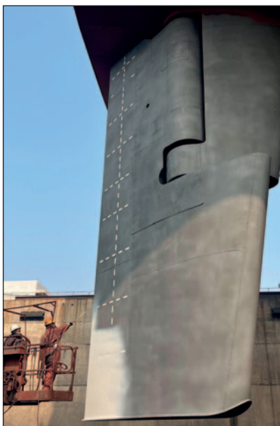
After surface preparation, Ecoshield is applied in two identical layers.
