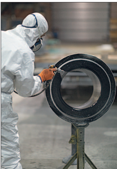
Ecoshield is chemically resistant, making it ideal for scrubber pipe protection.
