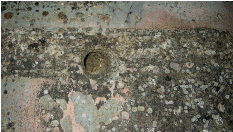
The Odyssey's hull before grit blasting and recoating in 2012.
