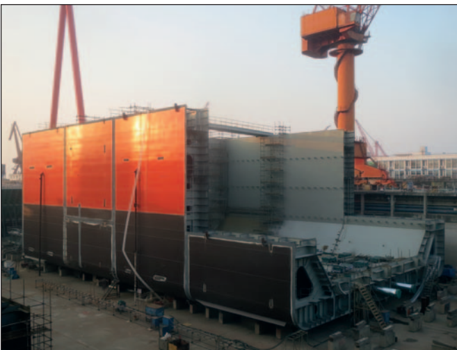
Large offshore units can be coated in the block stage. After assembly, erection joints and weld seams can be rapidly prepared and coated, forming one homogenous layer with earlier coated areas.
