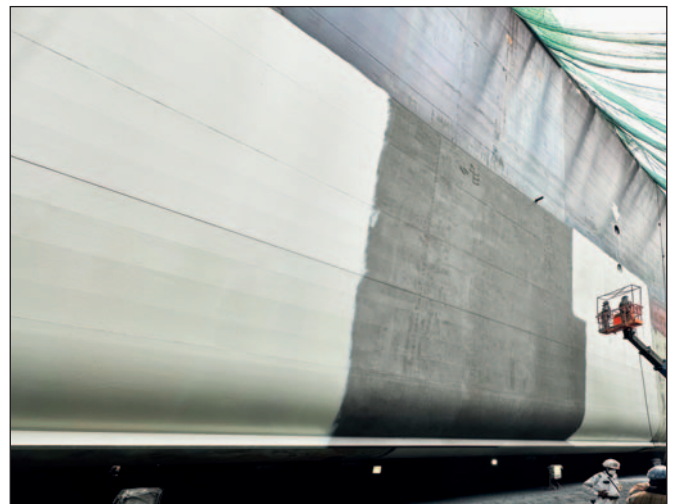
The second coat can be painted on with no limited window for application.
