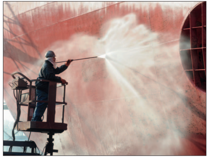
Cleaning can be performed underwater or with high-pressure washing in drydock without damaging the coating, maintaining efficiency throughout the vessel's service life.
