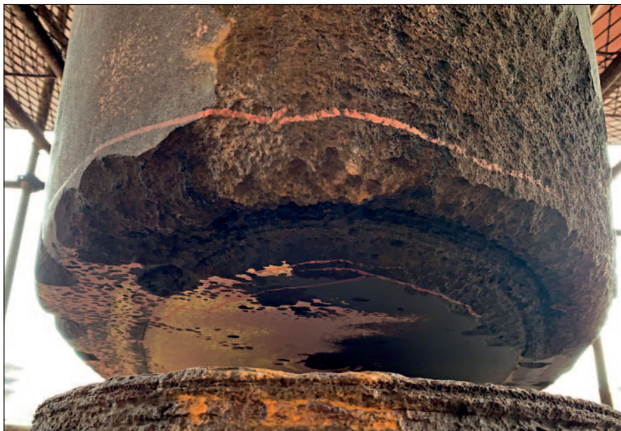
Severe cavitation damage on unprotected running gear highlights the limitations of conventional coating systems in high-impact zones.
