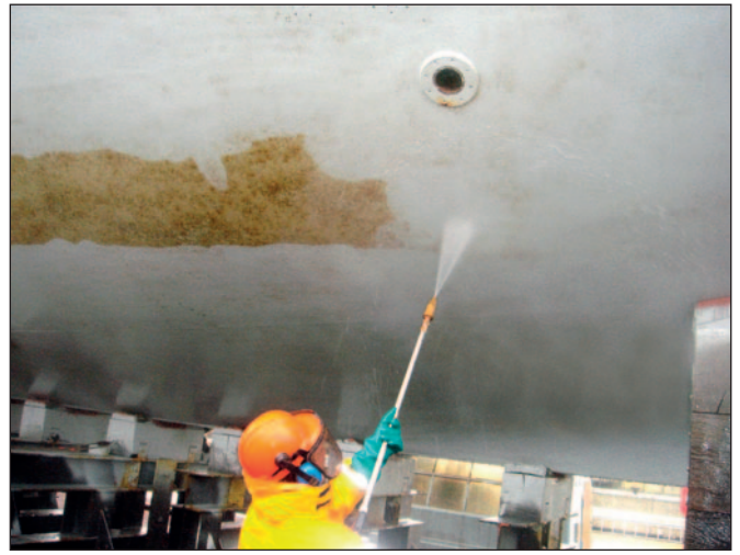
High pressure washing in drydock can also be done with the same result. No damage, no need to repair.
