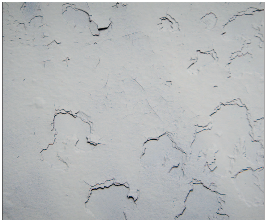
Hull of a ship where the antifouling coating has been "repaired" in drydock. This ship is about to undock.
