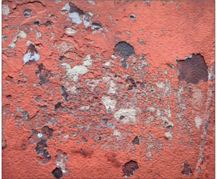
It is impossible to repair an antifouling coating that has degraded over time and restore the hull to a smooth finish.
