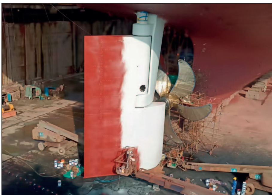
Ecoshield application is scheduled around other work on the vessel without interfering with it.
