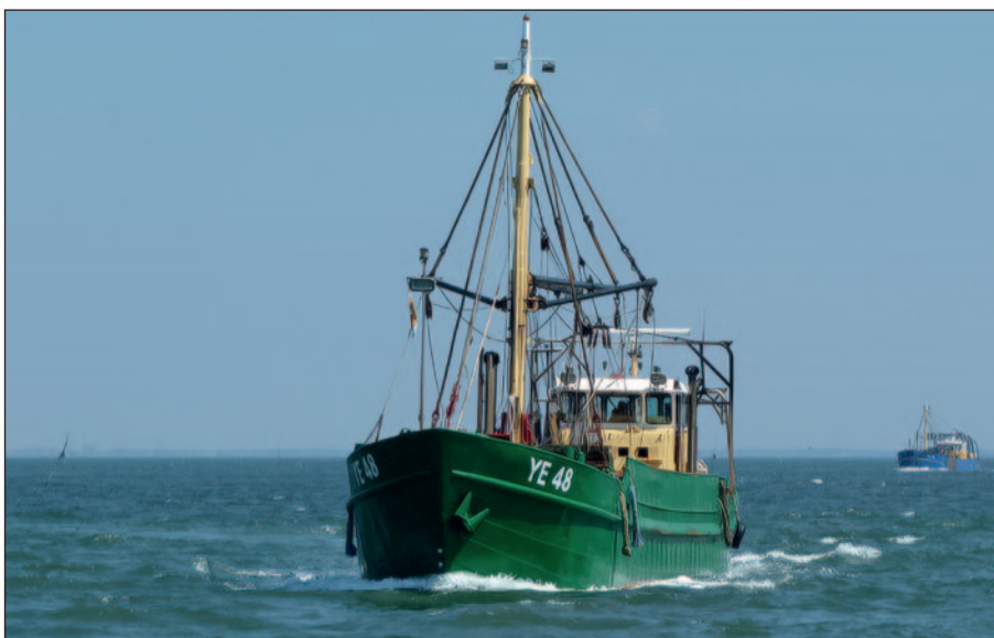
The oyster cutter YE 48 has successfully protected its hold with Ecospeed for 19 years without the need to repaint.
