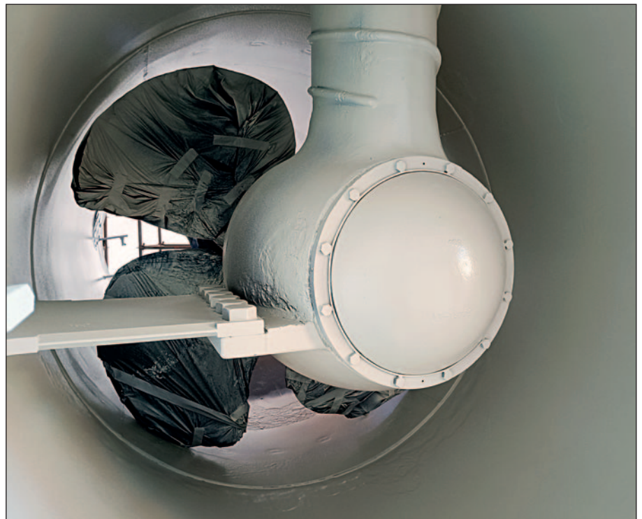
All running gear, such as thrusters and thruster tunnels, can be protected with Ecoshield.
