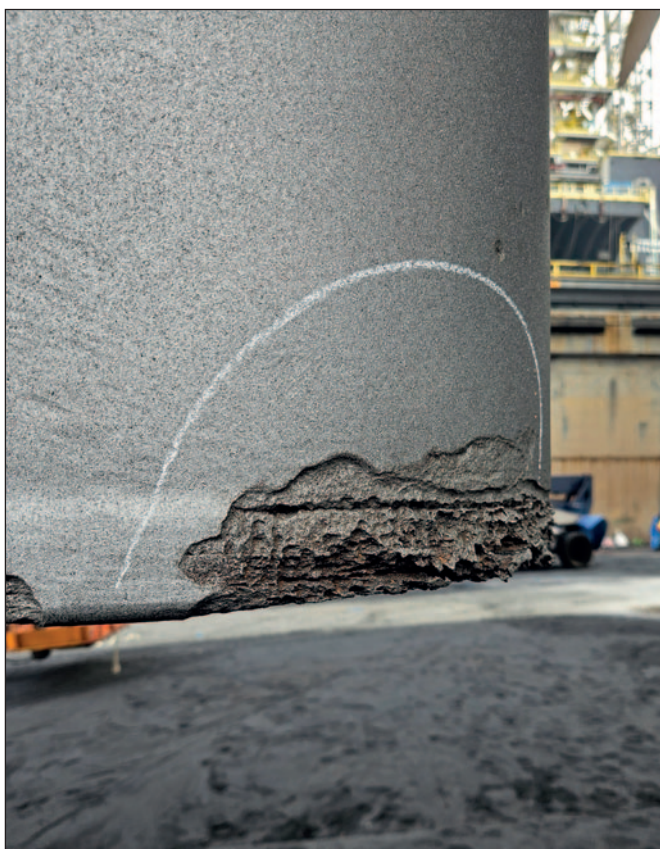
Severe pitting on rudder as a result of cavitation. Ecoshield can prevent this from happening
