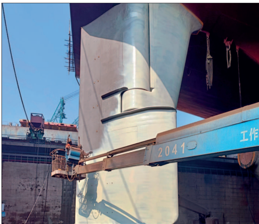
Ecoshield is applied in only two, identical layers.
