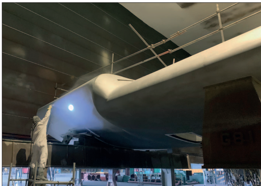
Ecoshield can be applied at the block stage, prior to installation of a rudder.
