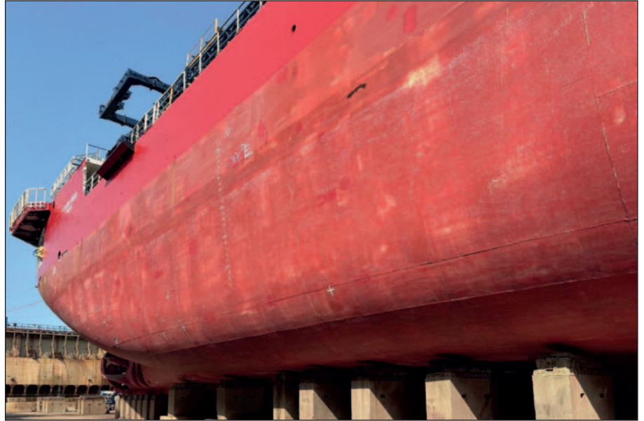
The coating on the vertical sides of the icebreaking research vessel Laura Bassi still looked amazing 16 years after first application.
