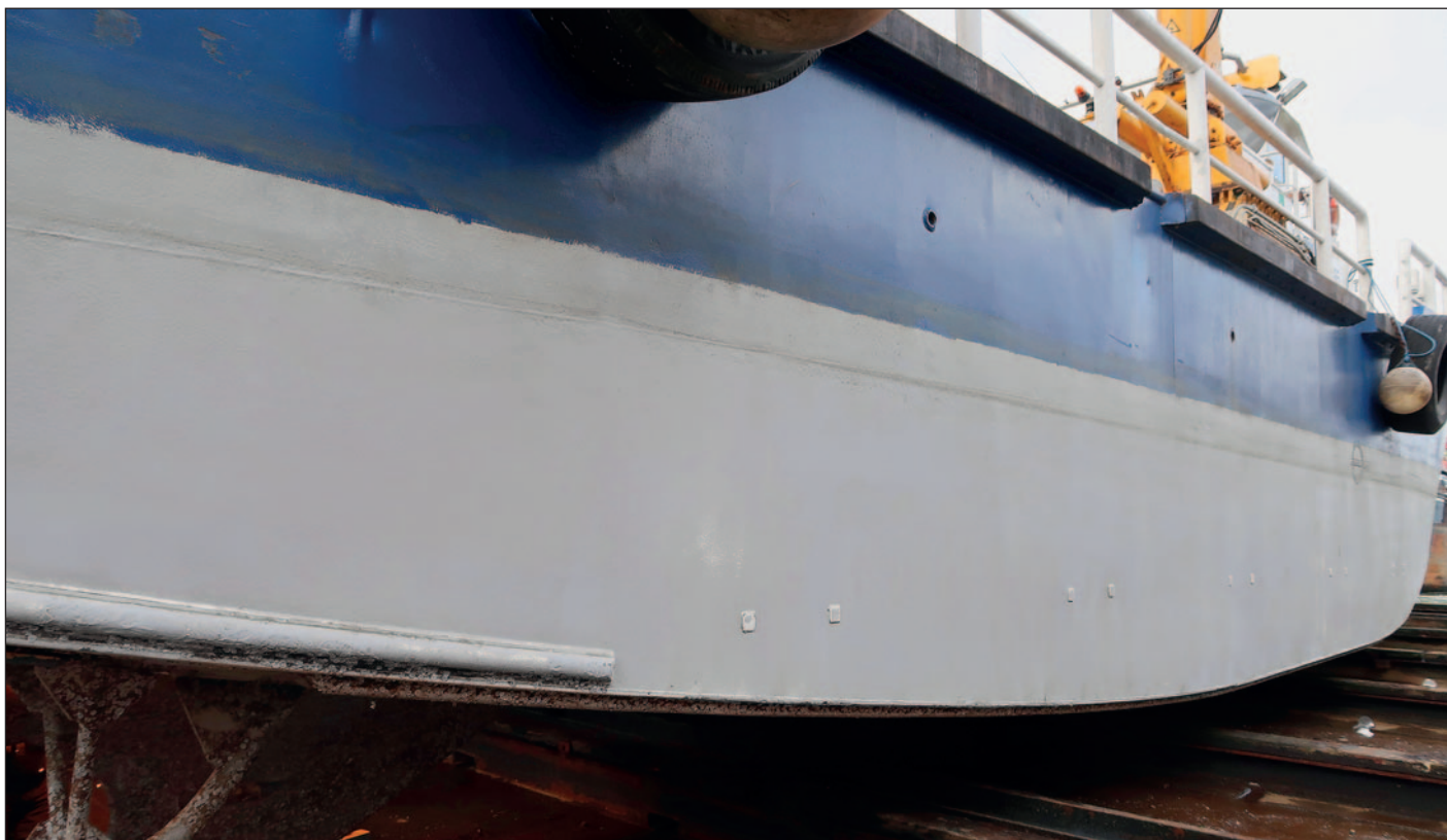
No repaint or touch-ups were required on this workboat after 10 years of sailing with Ecospeed.
