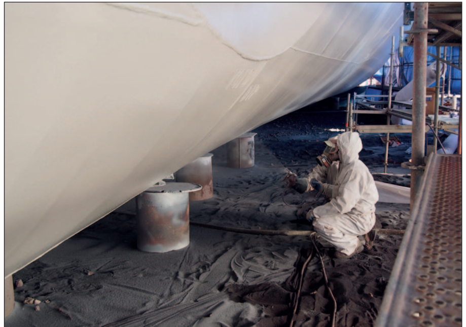
Ecospeed is applied in only two layers, no repaint will be needed during future dockings.
