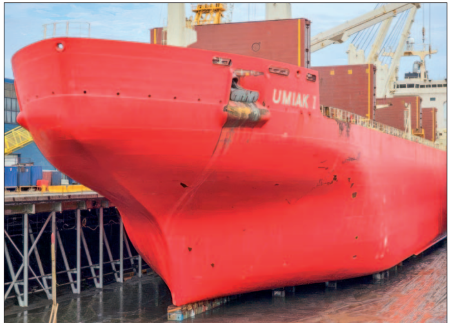
The Umiak I in 2024, showing no ice damage whatsoever three years after Ecospeed was applied to the hull.
