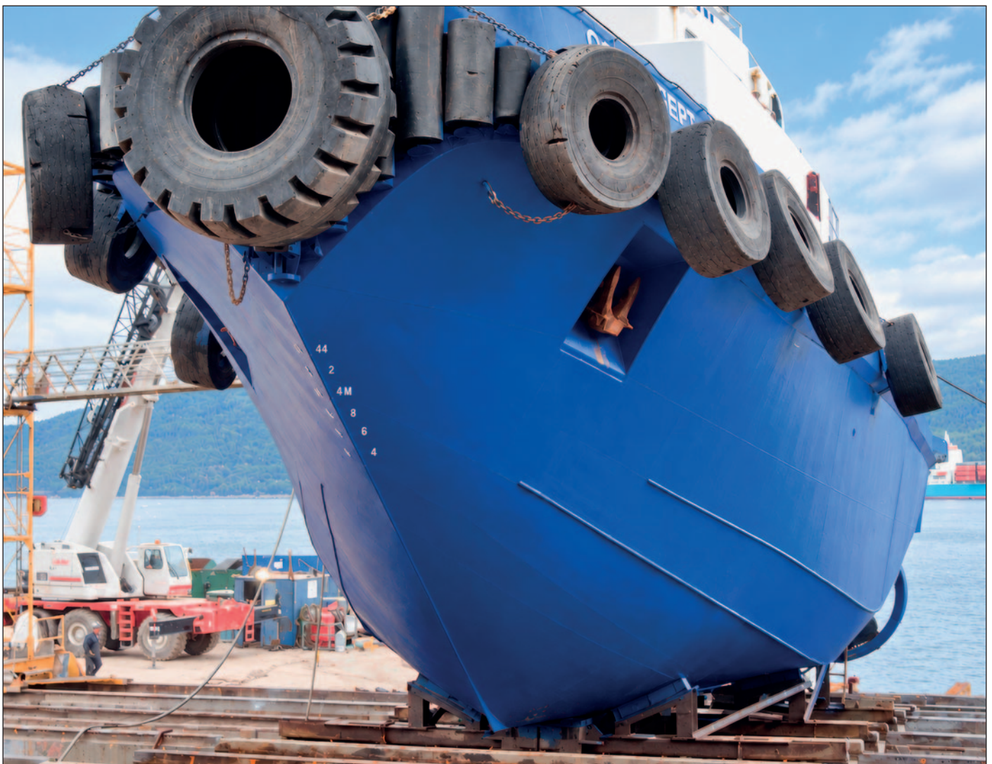
The Ocean Sept-Isles in drydock three years after Ecospeed was applied.
