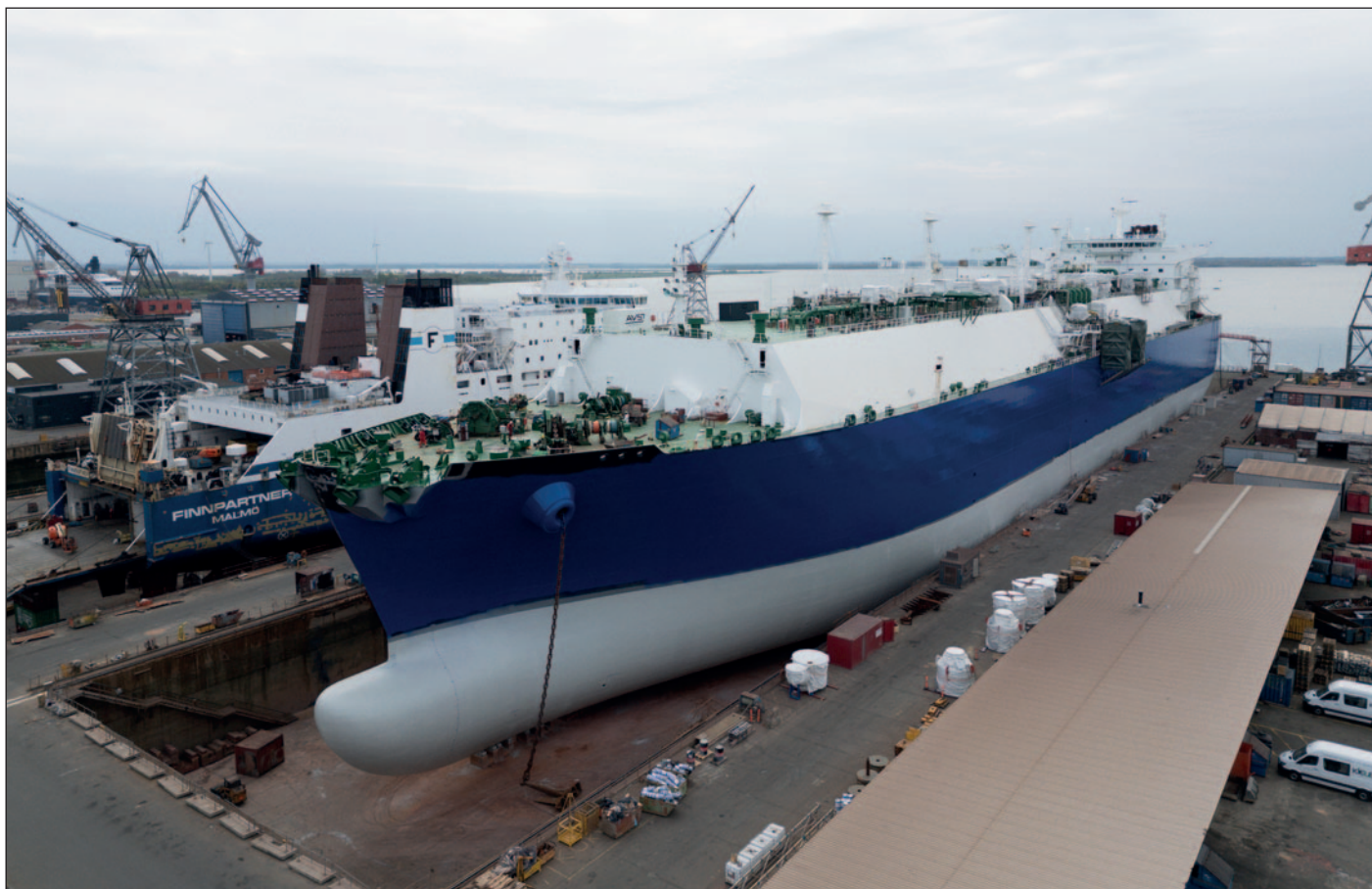
Newly converted LNG carrier to FSU in drydock recently coated with Ecolock on the underwater hull (grey).
