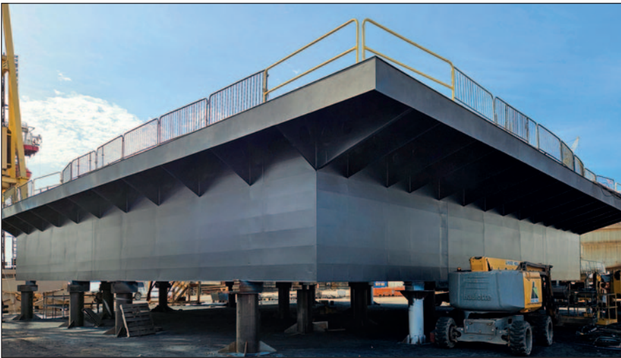
+ Pool test pool just coated with Ecolock, ready to go in the water.
