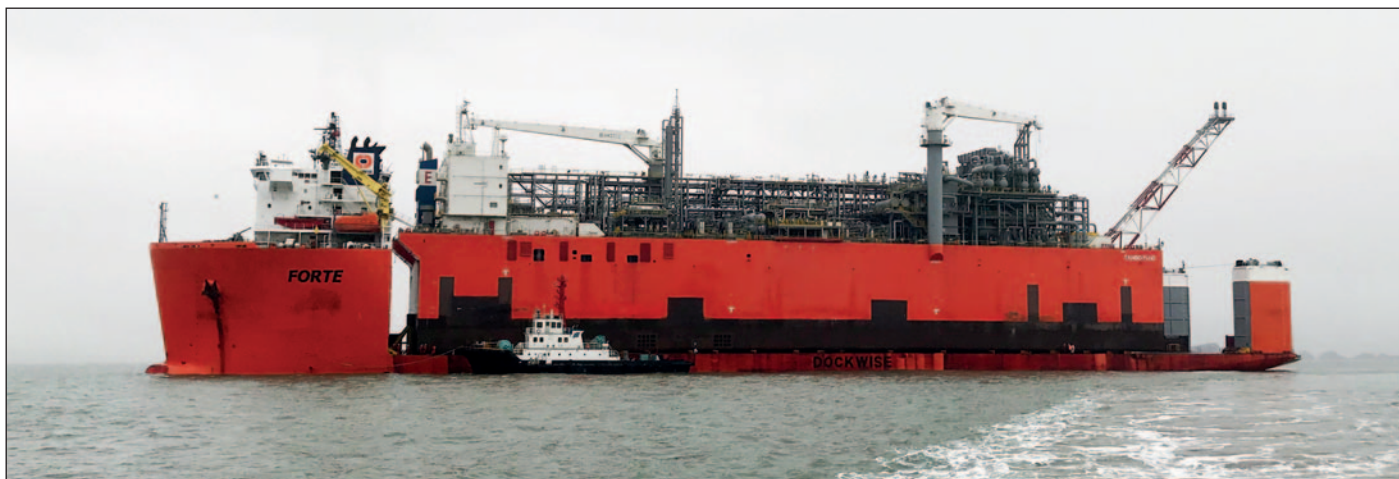
EXMAR's Caribbean FLNG renamed Tango FLNG en route to Argentina to take up station, the underwater hull and the fender areas coated with Ecolock.
