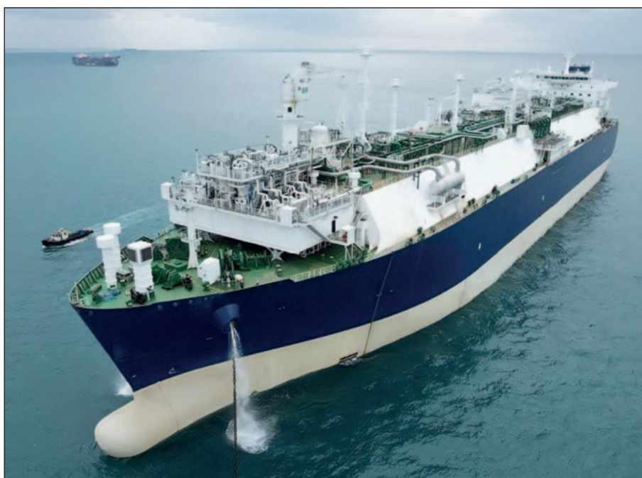
Recently converted LNG carrier, now an FSRU stationed off the coast of Brazil. The grey underwater hull, coated with Ecolock, was cleaned on departing Singapore for excellent fuel efficiency in the crossing.
